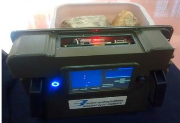
Figure 7. Setup for rescue applications for buried human targets
