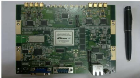
Figure 2. Multi-channel signal processing hardware [3]
